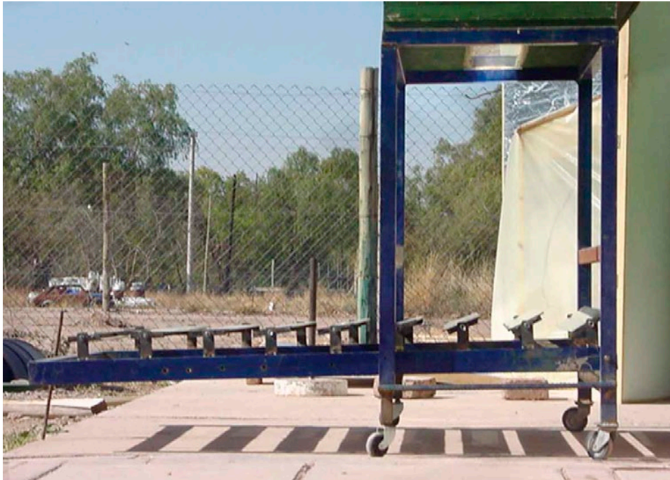
Fig. 5. Lower window with Fresnel reflectors in work position.
