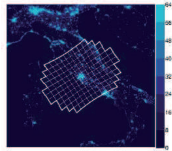
Figure 2: Observation area of JEM-EUSO telescope flying over central Italy. The background in the map shows visible light distribution obtained by DMSP data. The scales denote the values in DMSP units (see Section 3 for details).
