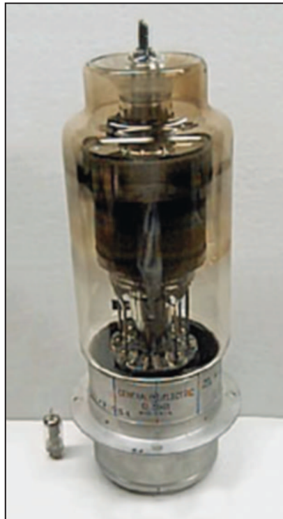
FIGURE 1 – A large GE thyatron (used in pulsed radars) next to a miniature 2D21 thyatron (used to control relays). (Courtesy of Wikimedia Commons.)
