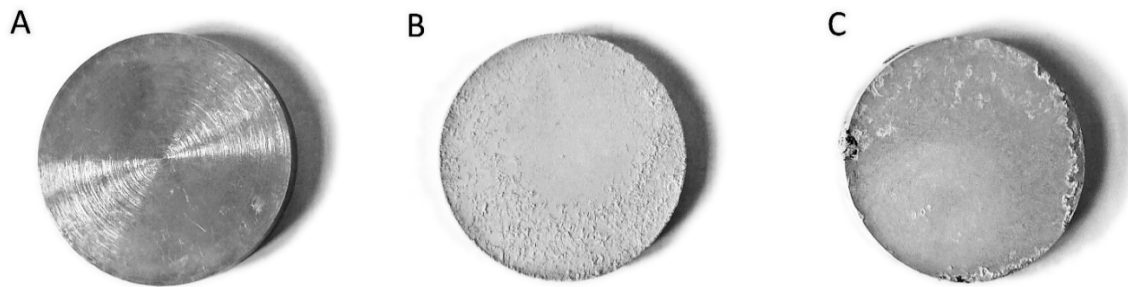
Figure 1. Stereo images of: (A) untreated sample; (B) sample PEO-Si; and (C) sample PEO-P.
