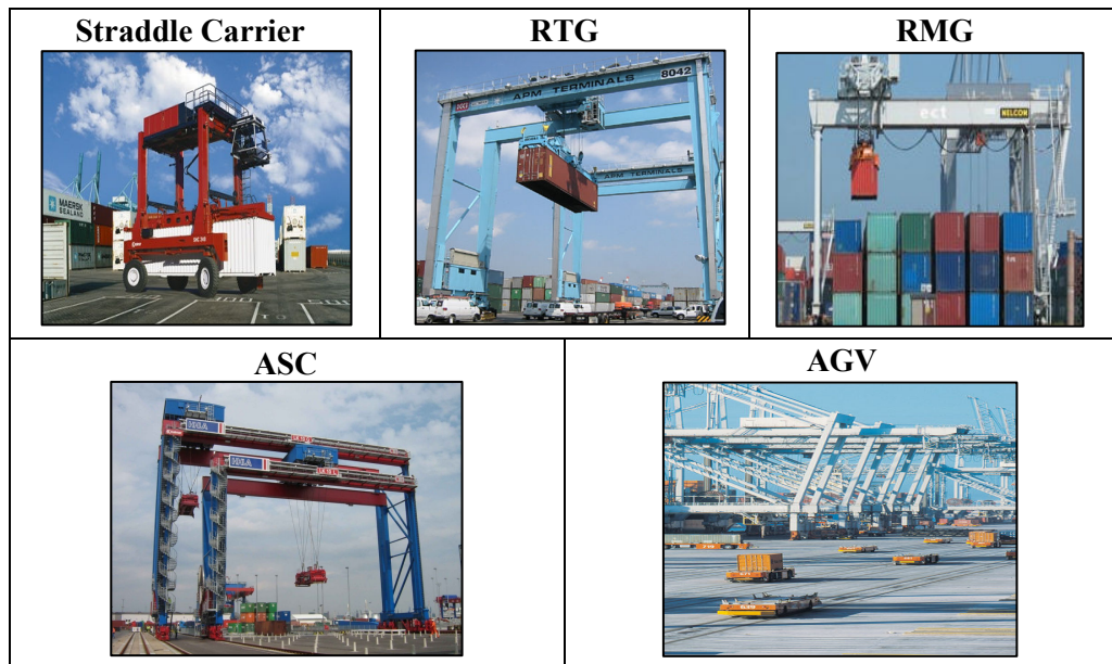
Figure 12: Main cranes and handling equipment used in the yard
