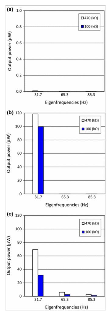
The bar charts in Fig. 16 compare the total output power from the converter prototype without an added mass (Fig. 16a) to that from the converter with an added mass (Fig. 16b). Each bar of the chart sums up the output power from each of the three transducers.
