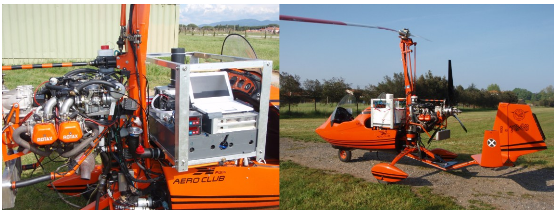
Figure 4.2: final configuration of AGRS_16.0L system.
