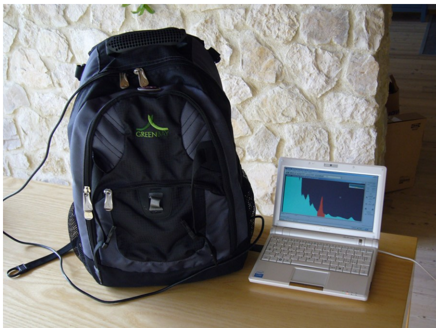
Figure 3.1: configuration of ZaNaI_1.0 system set-up in a backpack.
