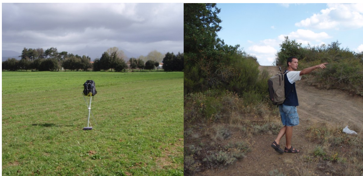
Figure 3.12: the tripod (static) and human back (dynamic) modalities of in-situ measurements.
