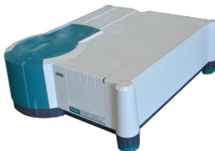
Figure 15: The UV-Vis spectrophotometer employed (Varian Cary 50). Wavelength range 190-1100 nm, maximum resolution 0.5 nm.
