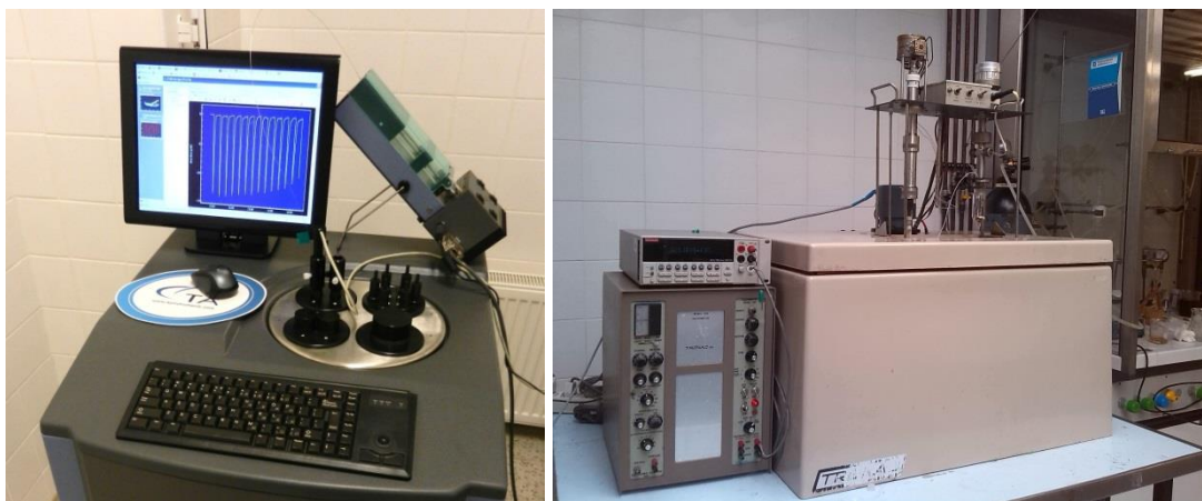
Figure 17: Calorimeters employed in this work. Left: Isothermal titration nanocalorimeter (TAM III), cell capacity 1 mL, sensibility > 10^{-5} J; right: isoperibolic titration calorimeter (Tronac model 87-558), cell capacity 25 mL, sensibility 1 J.
