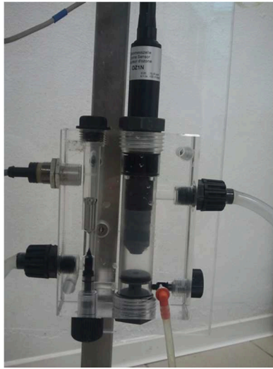
Figure 6. 2 Ozone analyser and tank with sample, from the bottom to the top respectively
