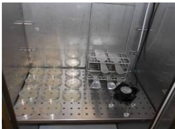
Figure 4.2 The internal chamber for gaseous ozone treatment.
