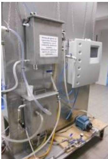
Figure 4.3 The plant for aqueous ozone treatment.
