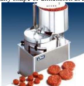
Figure 5.1 The MS-automatic moulding machine for hamburgers (Nilma, 2012).
