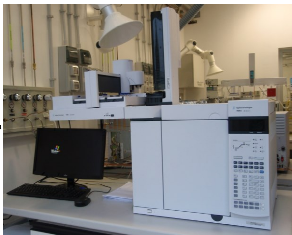
Figure 24. Scheme of MOSH and MOAH elution from a SPE cartridge packed with silvered silica (left) and GC-FID 7890A system (Agilent Technologies) used for a large volume injection (right).
