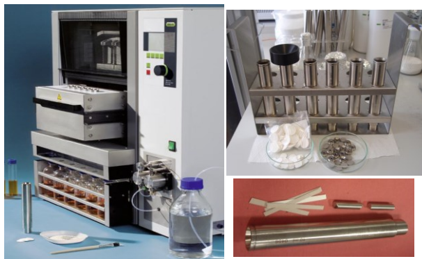
Figure 33. Pressurized Liquid Extractor from Büchi; 10-mL stainless steel extraction cells with cellulose filters, metal frits and 2-mL expansion elements.
