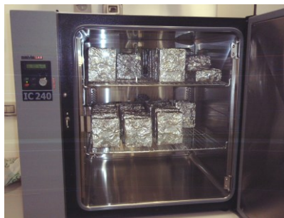
Figure 67. Thermostat (Incucenter IC240, SalvisLab) containing pasta packs wrapped in aluminum.
