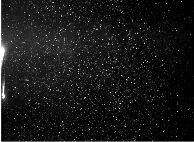
Figure 2.4: Sample streamwise PIV image at Re = 10000 . Pipe outlet is visible at the far left of the picture.
