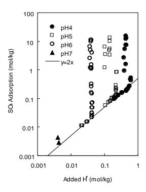
**Fig. 1.** Sulfate adsorption and added protons to maintain constant pH in the adsorption experiment. A  $H_2SO_4$  solution was added for the pH adjustment.
