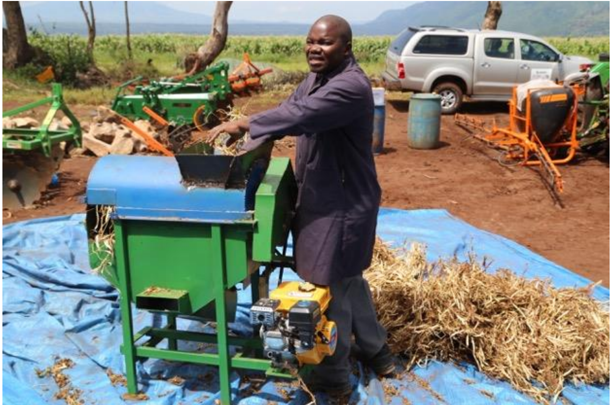
This bean shelling machine prototype and other technologies will also be part of the array of improved technologies that will be demonstrated for farmers at Mushobozi's farm. This shelling machine prototype which (still is being enhanced) uses 0.3 litres of petrol to thresh 295 kg of beans/hour. This translates to a labour saving of 73% when compared to manual threshing of beans. The machine is seven times more efficient compared to manual threshing (photo credit: Jonathan Odhong'/IITA).
