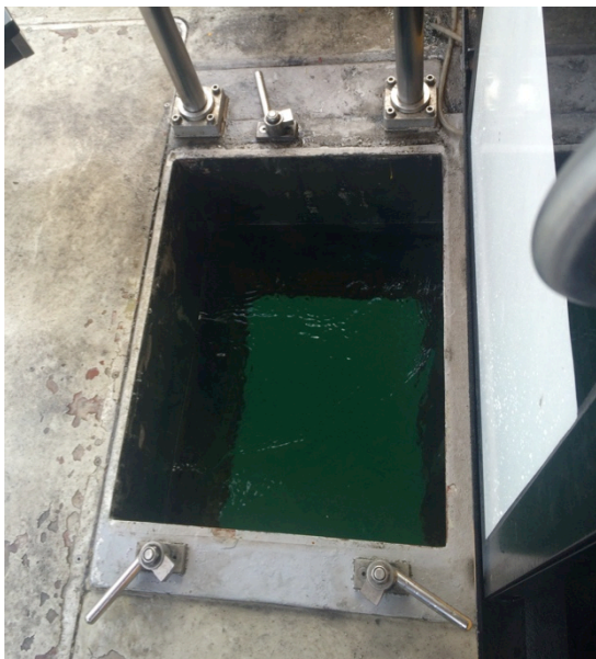
Figure 15: Hole on the boat for the sounder – Own source
