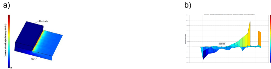
Figure 10. a) Current density in a simulated electrical connection to a CFRP coupon (adopted from Romero et al., 2014); b) Distribution of the potential difference between two faces of the coupon in Figure 10 (adopted from [30]).
