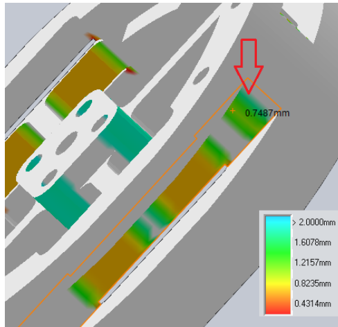
Figure 3-9. Thick analysis for 25° between fixing holes
