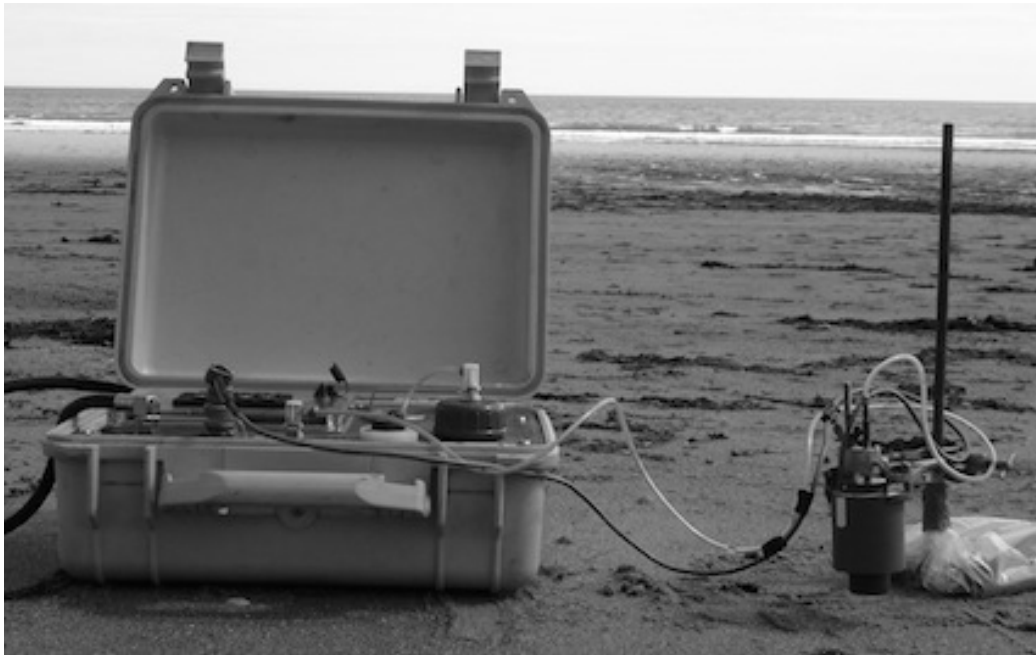
Figure 2.6: The Cohesive Strength Meter erosion device.
