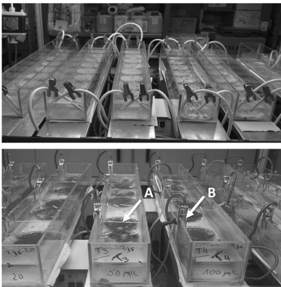
Figure 7.1: Experimental setup: Prior to experiment (top) and during experiment (bottom). Triclosan rods and air pump system are marked with A and B respectively.
