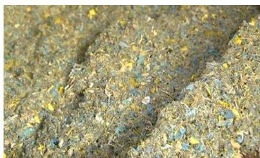
Figure 6-11. Shredded and unrecognisable microwaved healthcare waste
