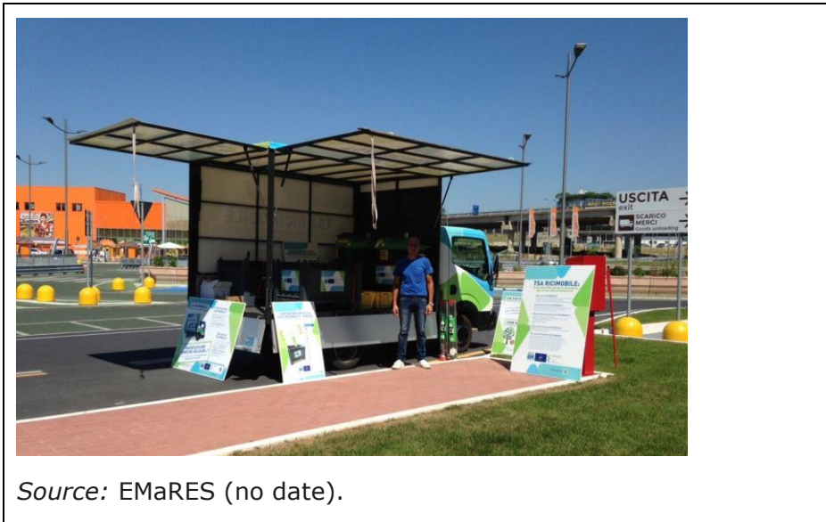
Figure 4-36. The Dynamic Ecopoint "Ricimobile", a 7.5-tonne vehicle for the collection of small WEEE, used cooking oil and batteries
