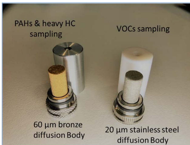
Figure 7 - PoD sampler with different diffusion bodies for PAHs and VOCs sampling
