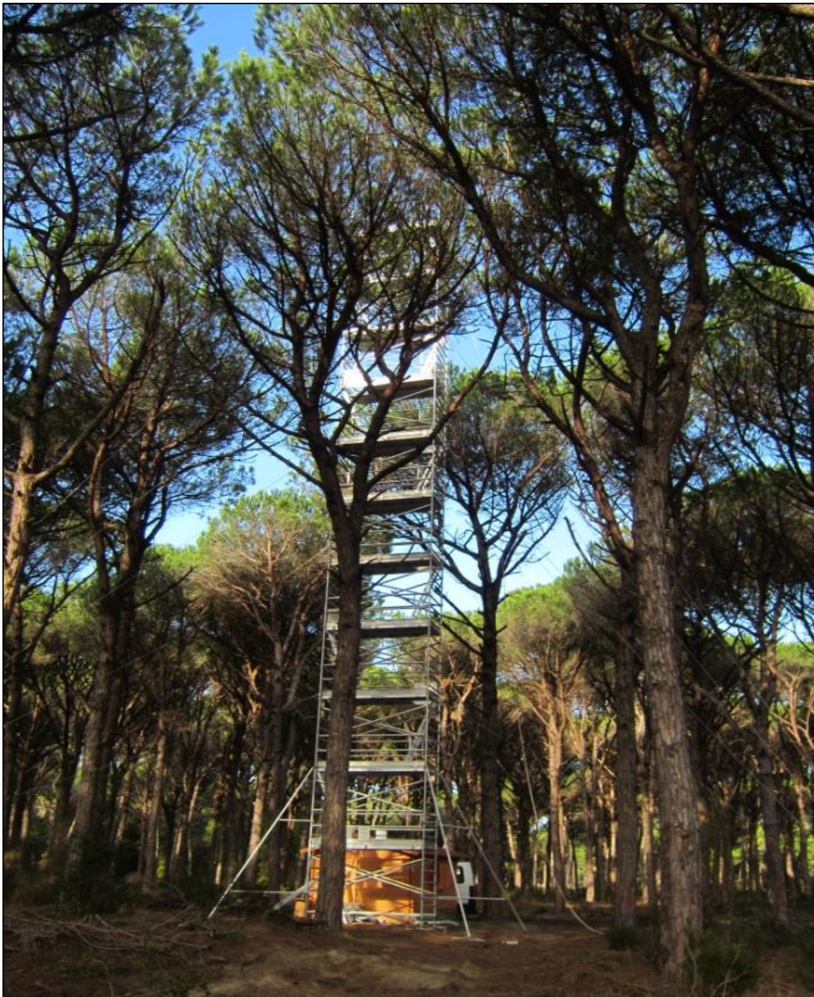
Fig. 54: the flux tower of 24 m at the Pinus pinea site in San Rossore
