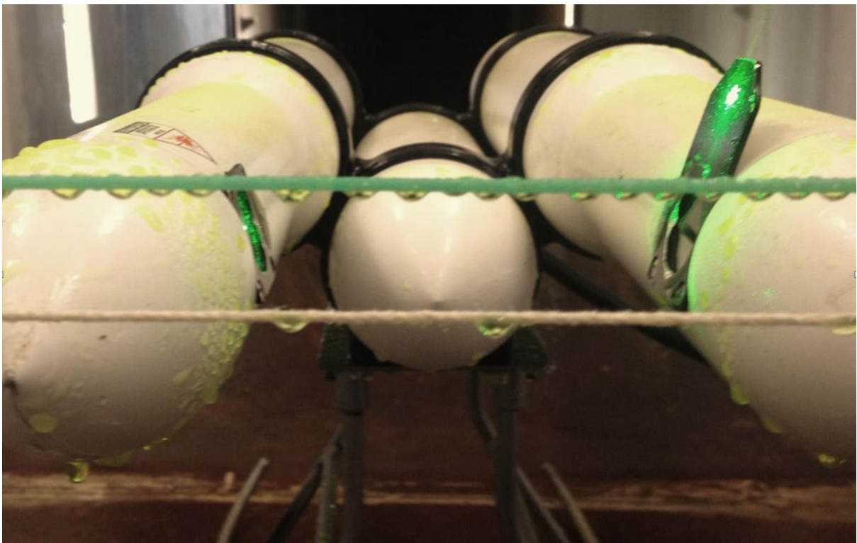
Figure 4.4 Illustration of saturation and droplet accumulation on nylon (upper) and cotton (lower) strings.
