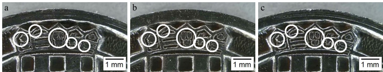
Fig. 5. Geometry details of the coin with different crystalline grain size a) 25 \mu\text{m} , b) 50 \mu\text{m} , c) 90 \mu\text{m} , obtained with 150 kN forging force
