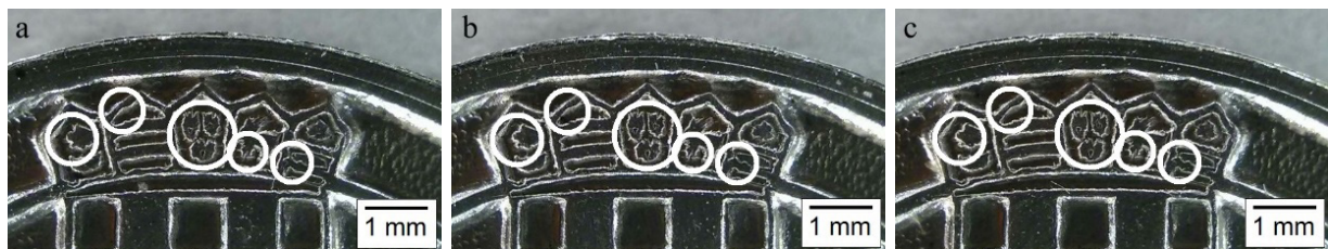
Fig. 6. Geometry details of the coin with different crystalline grain size a) 25 \mu\text{m} , b) 50 \mu\text{m} , c) 90 \mu\text{m} , obtained with 200 kN forging force
