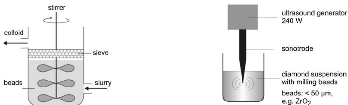
Figure 8: Schematic of bead milling method (left) and bead assisted sonic integration (right) [60].
