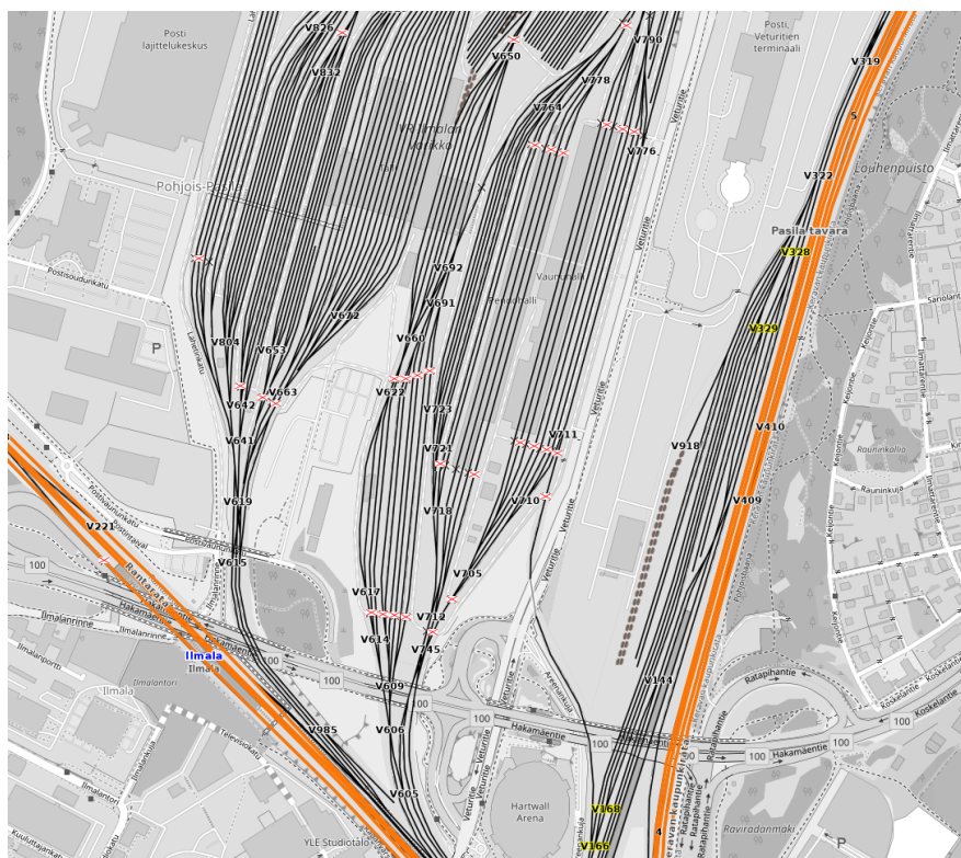
Figure 1.1: An overview of Ilmala rail yard. The different railway switches are marked V619, where 619 is the switch-specific number of that area. A detailed location of the different switches used in this thesis can be found by zooming in on the Ilmala area on the Open Railway Map web pages 2 .
