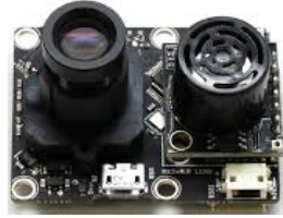
Figure 2.2: Optical Flow sensor with CMOS image, gyroscope and ultrasonic[34]
