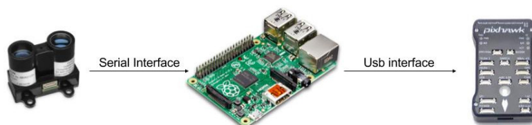
Figure 6.5: Integrate obstacle avoidance with Garmin Lidar
