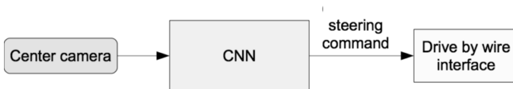
Figure 3.3: Deploying End to End FCNN for autonomous driving [9]
