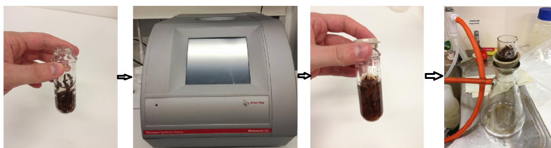
Figure 27: Experimental set-up of hot water extraction with microwave reactor.
