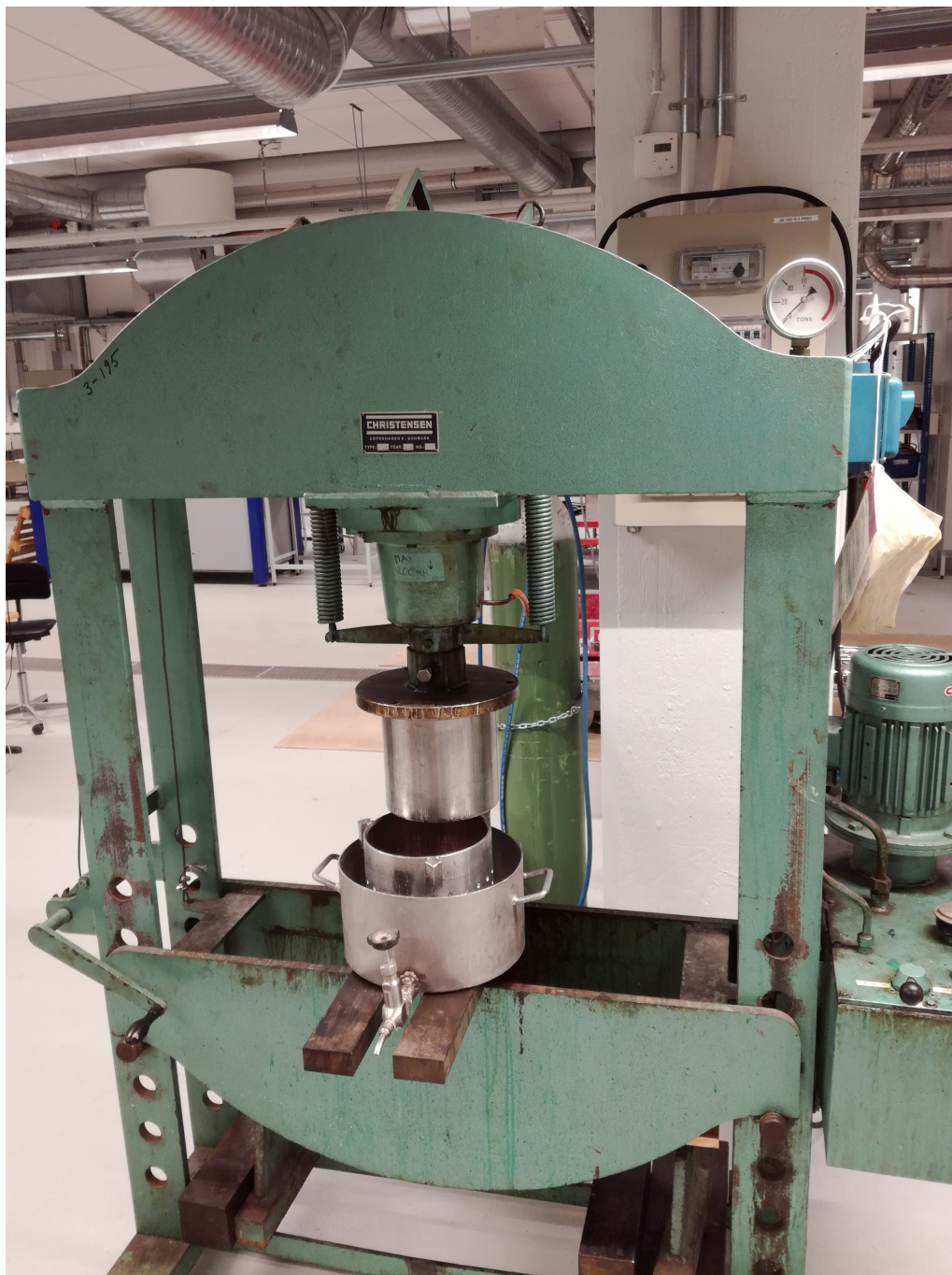
Figure A1: Mechanical press applied to press spruce bark after steam assisted extraction of water soluble extractives.
