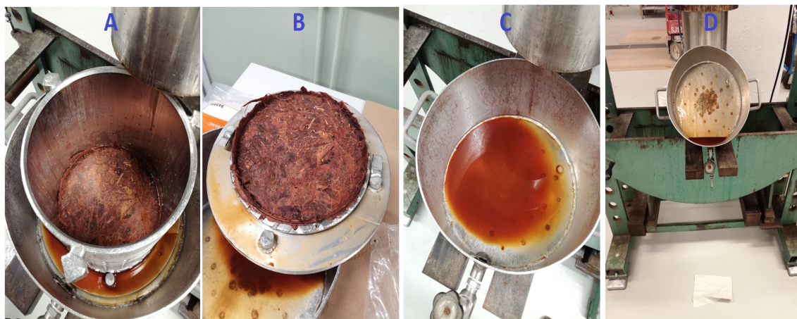
Figure A2: Disassembling the pressing vessel: (A) Removing the pressing piston; (B) removing the plate holding the bark; (C and D) collecting the extracts in a container.
