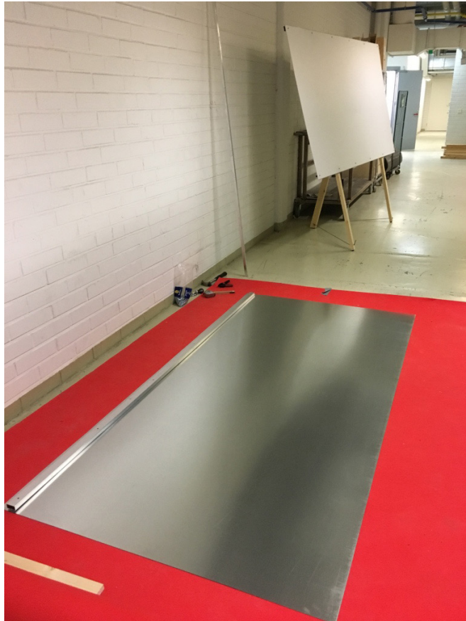
FIGURE 36: IN THE FRONT, ALUMINIUM PIPES ARE TO BE ATTACHED TO THE BACK OF A PATHWAY BOARD. IN THE BACK OF THE PICTURE IS A FINISHED BOARD ON A STAND.
