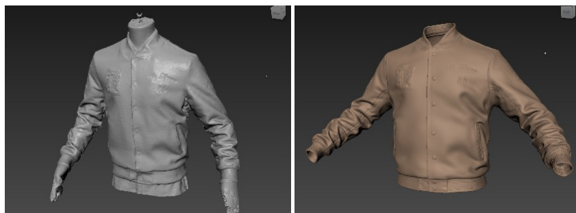
Figure 40 Scanned jacket and the same garment after cleaning and re-sculpting. The sleeve is pulled up slightly to form small wrinkles on the arm. (Huovinen et al., [no date]: 12)
