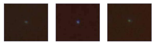
Figure 3.14: Silver nanoparticles held in a single beam trap with 40nm, 60nm and 80nm diameter (from left to right). The scattered light from the nanoparticle increases with size. The colour of the silver nanoparticles changes from blue to green due to the redshifting of the resonance for larger particle sizes.
