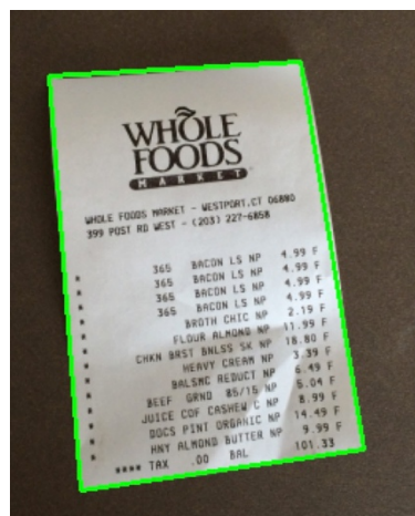
Figure 6 - Source image with detected contour in green. Source: (Rosenbrock, 2014)
