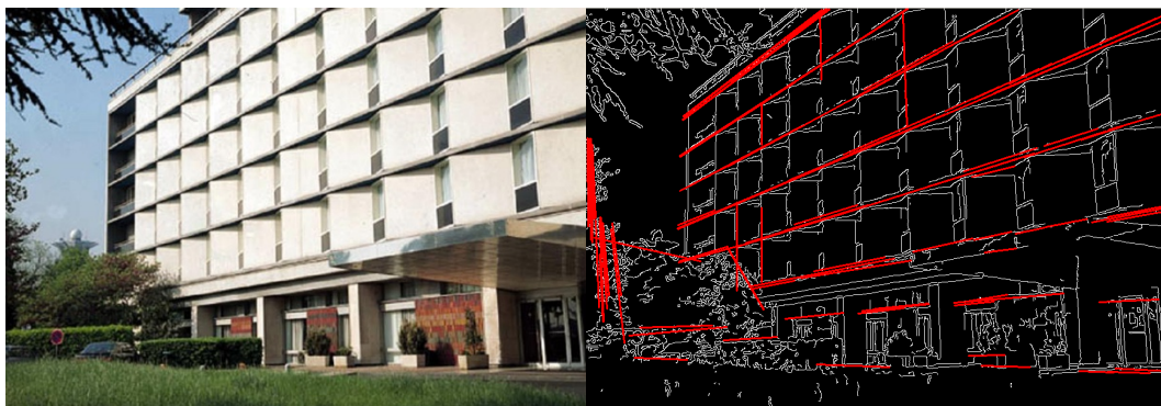
Figure 7 - Using the Hough transform to find the vanishing point of an image. Source: (OpenCV, 2017)
