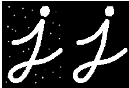
Figure 35 - Original image, left. Opened image, right. Source: (OpenCV dev team, 2014)
