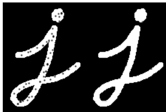
Figure 36 - Original image, left. Closed image, right. Source: (OpenCV dev team, 2014)
