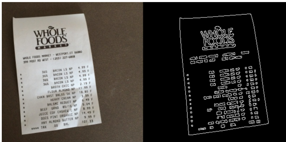
Figure 5 - Original image, left. Image after Canny edge detection, right. Source: (Rosenbrock, 2014)
