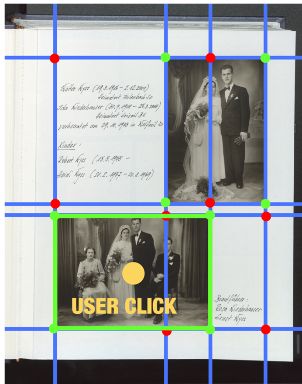
Figure 19 - Illustration of the process detecting lines and corners, and determining the image based on user click position
