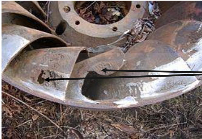
Figure 2.5: Worn out impeller [Courtesy of Turbine Francis].
