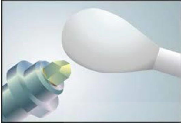
Figure 2.20: Indenter cleaning by cotton swap [www.microstartech.com]
