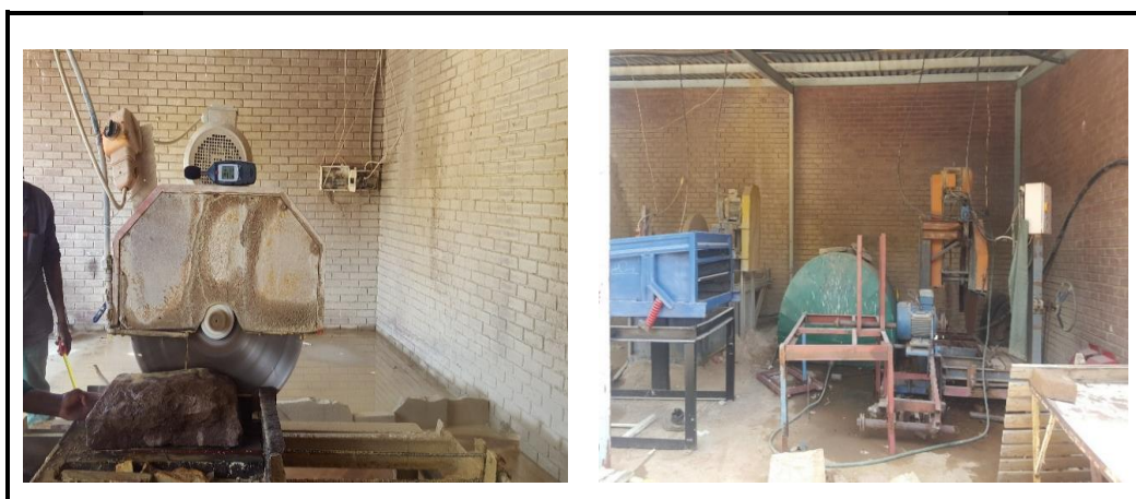
Figure 54: Illustration of the cutting of sandstones as performed at the processing plant
