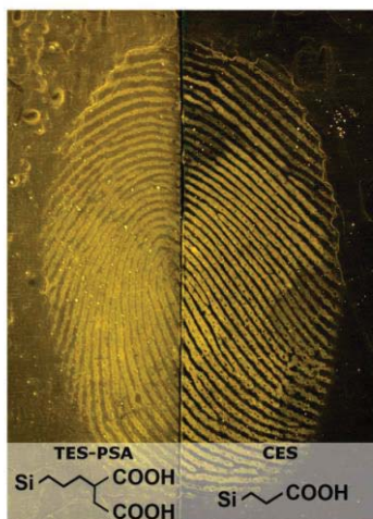
Figure 3: Comparison between Rhodamine 6G-doped silicon oxide nanoparticles functionalised with TES-PSA ((triethoxysilyl)-propylsuccinic anhydride – left half) and CES (carboxyethylsilanetriol – right half), and used to detect fingermarks. The illustrated fingerprint is one-week old, deposited on aluminium foil and visualised in luminescent mode (excitation at 495 nm and emission at 590 nm).
