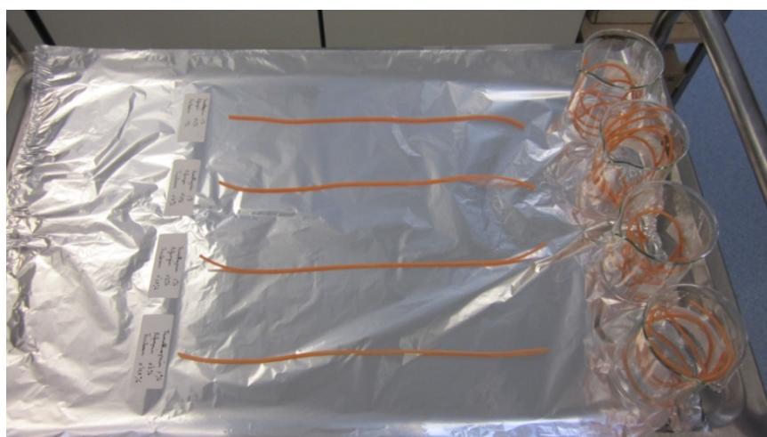
Fig 4. Silicone-impregnated tubing with 0.2% rifampin, 1% trimethoprim and 1% triclosan. The original white tubing turned orange due to rifampin.
