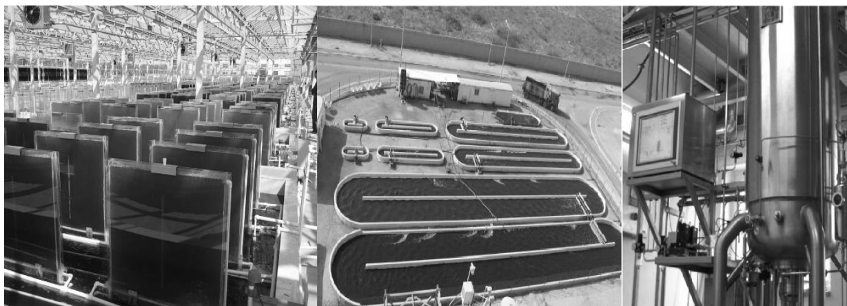
Figure 7 A plated bioreactor, an open raceway pond and a traditional fermenter all considered to be potential ways to mass cultivation of microalgae
