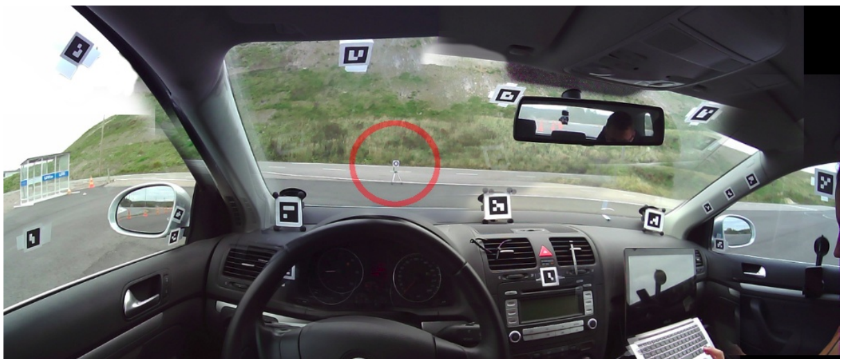
Figure 8. Test track car interior from driver's point of view. Markers are for 3D model identification to determine the horizontal axis of the car. Calibration target marker can be seen on a tripod in front of the car, highlighted by a red circle.
