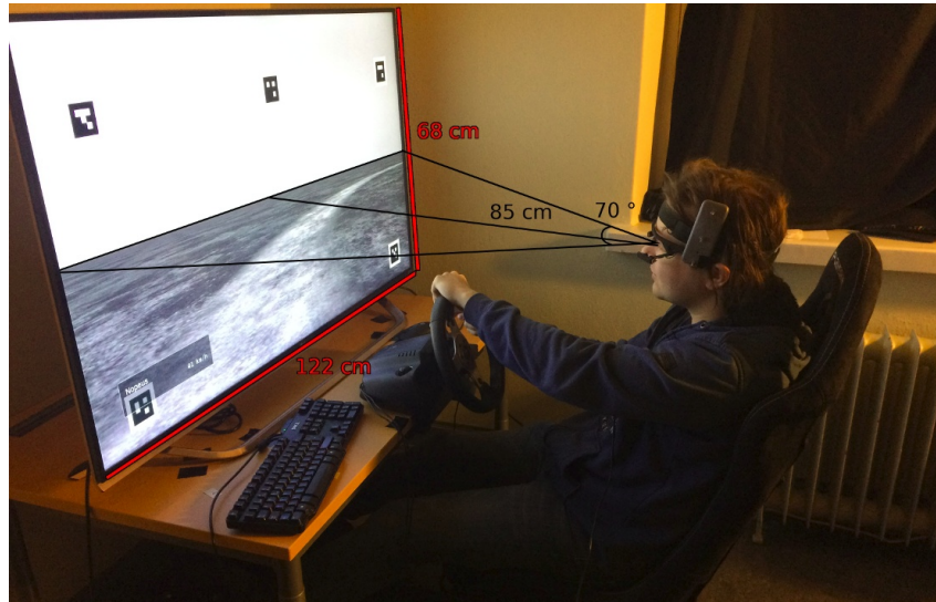
Figure 6. The physical setup of the simulator. The room's lights were turned off during the actual test. Keyboard was used for typing background information.
