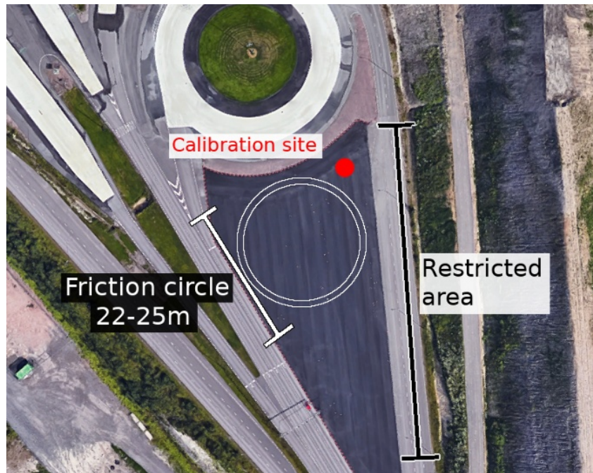
Figure 9. Double circle drawn to the map indicates the test track painted on the asphalt. (Google maps, 19.3.2018)
