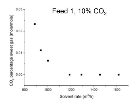
Run absorber hard to get 50 ppmv  $CO_2$  for LNG prep. (vs 2% pipeline gas)
