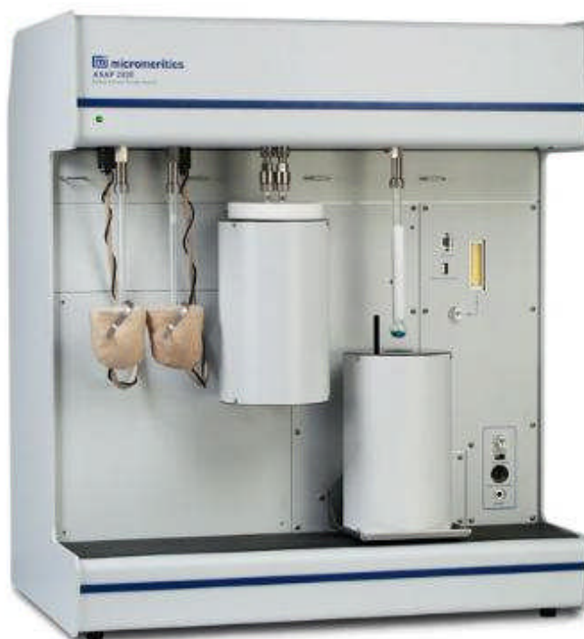
Figure 3.9 A Micromeritics ASAP 2020 Surface Area and Porosity Analyser. Degas ports are on the left complete with heating manifolds. The analysis port is on the right with a liquid N 2 bath directly below.
