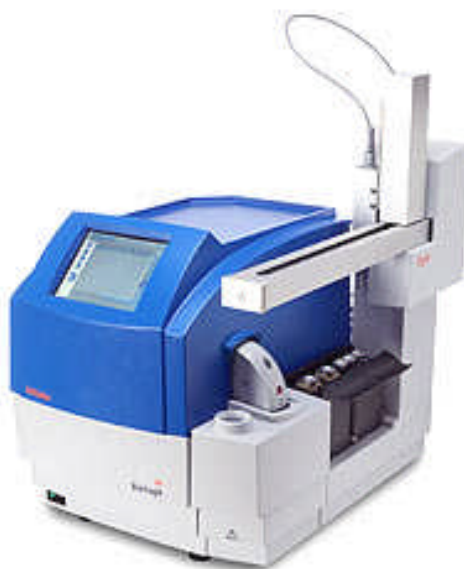
Figure 3.1 The Biotage Initiator Eight 12 used for all microwave experiments mentioned.
