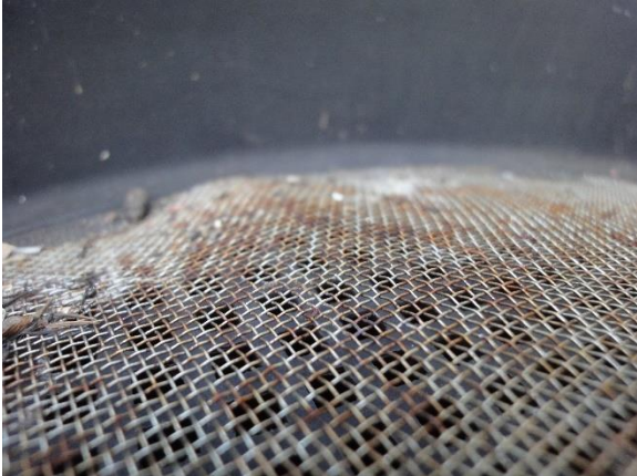
A13. Sieve degradation through rusting, manufacturing failure and intentional disruption (bottom two images).
