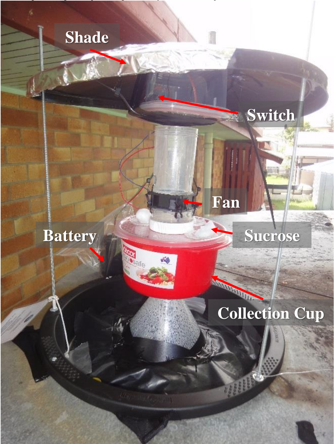
A10. Design of emergence trap including fan, battery and collection cup.
