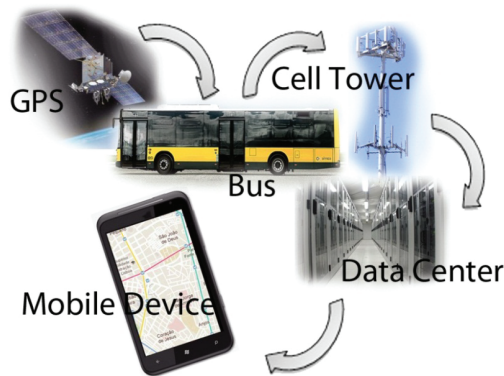
Figure 3.5: NextBus Architecture (figure from [3])
