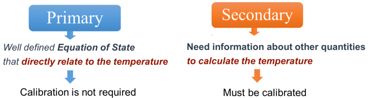
Figure 1.2 Types of thermometry: primary and secondary.
