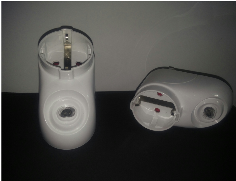
Figure 4.2: Two smart plug prototypes used in the proof of concept, also provided by WithUs Lda.
