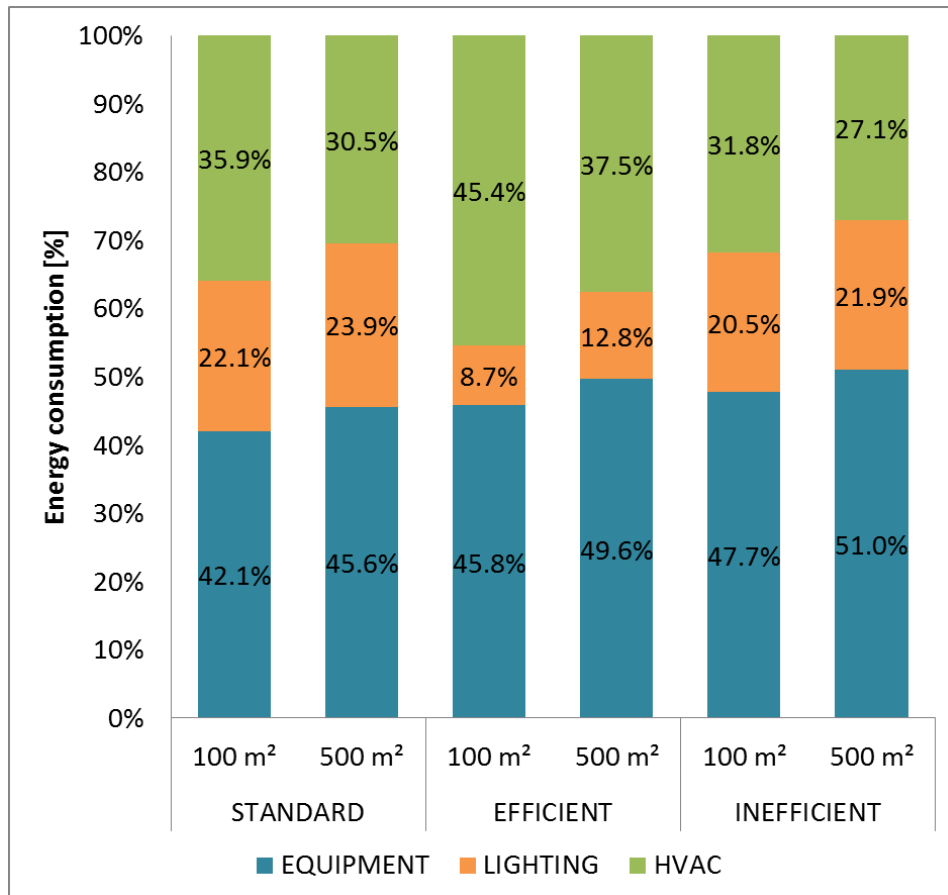
Figure 15: Energy consumption by category, size and occupant profile, in relation to standard occupants.
