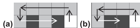
Figure 6. Moving loads with different amount of interspace: (a) one interspace, (b) no interspace.
