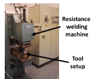
Figure 2: Electrical resistance welding setup.
