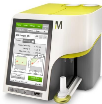
Figure 3.3 A picture of the “muse”, a small table top flowcytometer that was used to obtain the data in the \gamma H2AX assay Figure taken from [106]
