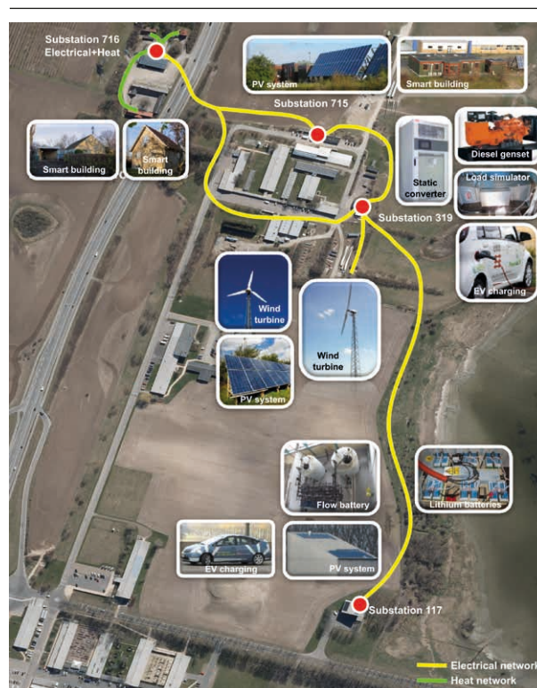
Figure 5. The importance of being able to test microgrid solutions under real or semi-real conditions, as in DTU's SYSLAB experimental research facility (illustration: DTU 2018).
