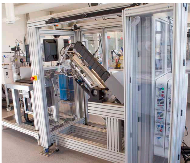
Figure 3. High pressure unit for fluid phase behavior study at DTU
