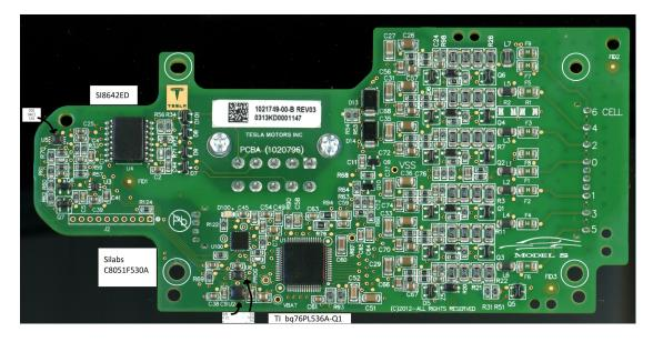
Figure 2.2: Tesla Model S 85kWh BMS PCB [1]
